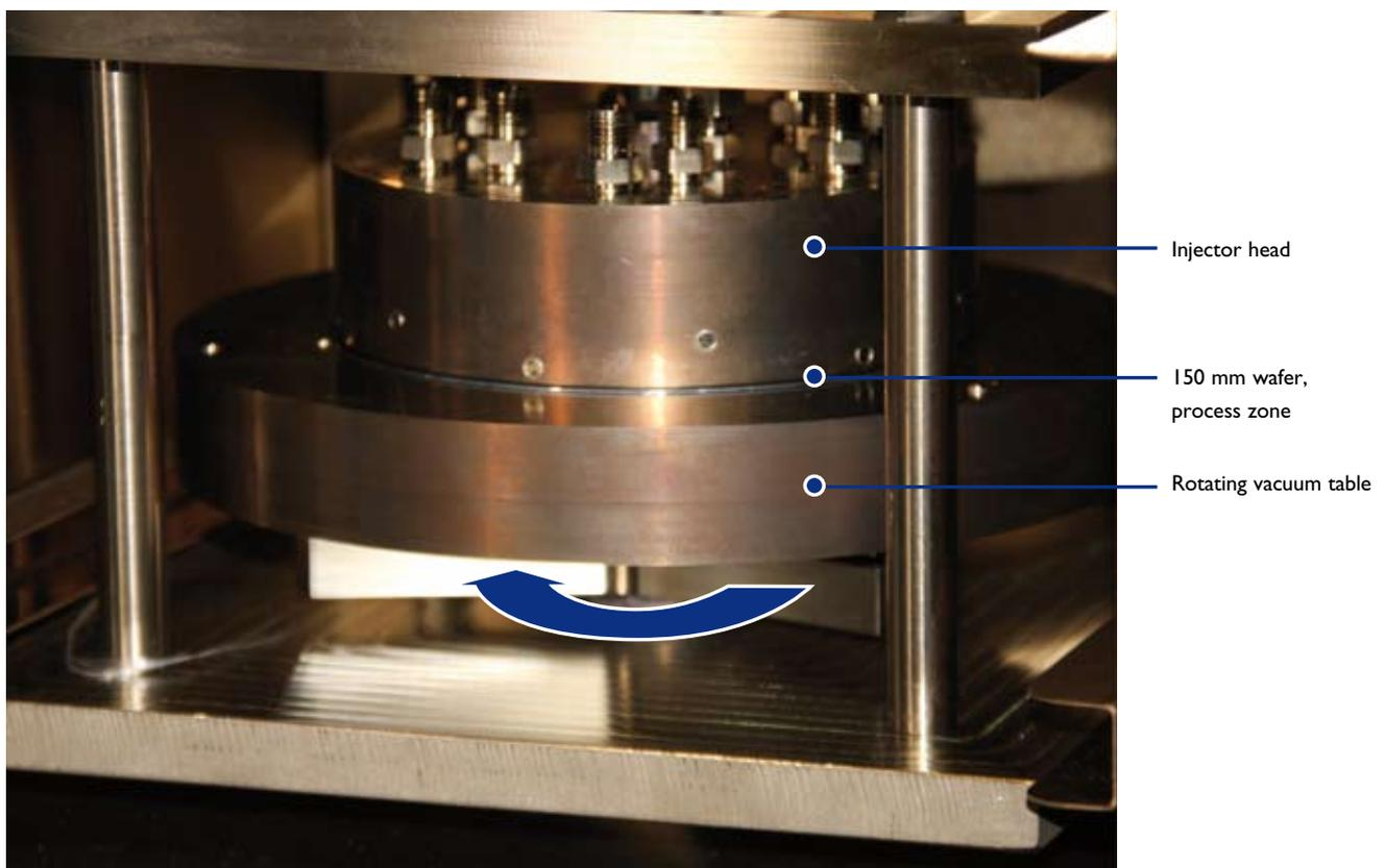
Figure 2. The ALD reactor for 150-mm substrates.
