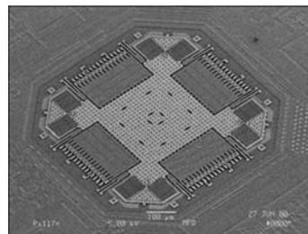
Figure 1. MEMS accelerometer commercialized by Analog Devices in airbags and game consoles.
