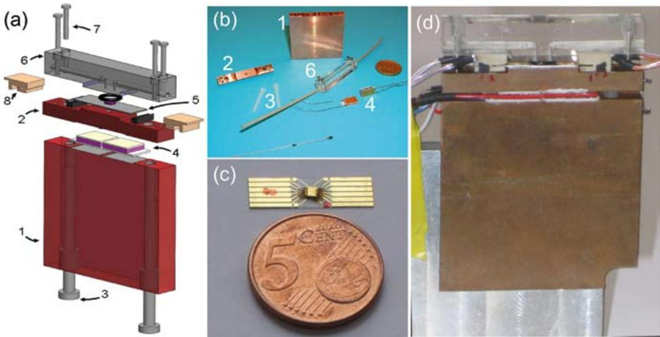
Figure 7. Construction of a flow cell.
