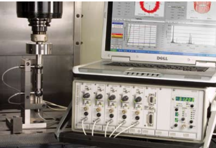
Figure 4. Double-ball set-up for IBS's Spindle Error Analyser.
