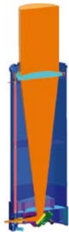
Figure 3. The Optical Tube Assembly expands a 15 mm input laser beam to a steerable 300 mm output beam.
