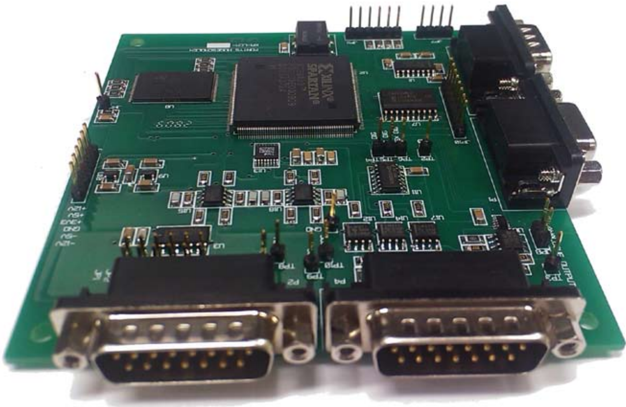
Figure 5. The final result: a high-end, low-cost motion control board.
