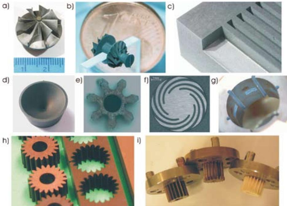
Figure 7. Application examples of ceramics and ceramic composites manufactured by micro-EDM.
