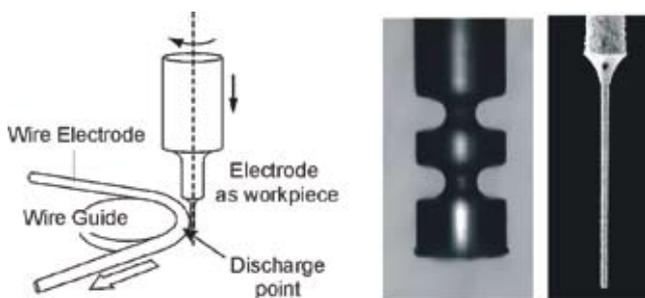
Figure 3. Schematic view of WEDG (Wire Electro-Discharge Grinding) and examples of shaped tool electrodes  $\varnothing 0.3 \text{ mm}$  (left) and  $\varnothing 20 \mu\text{m}$  with aspect ratio of 20 (right).
