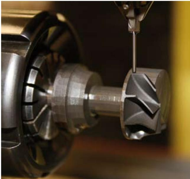
Figure 8. Three-dimensional micro-EDM milling of a  $\text{Si}_3\text{N}_4$ -TiN turbine impeller in progress.
