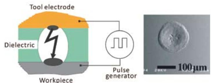
Figure 1. The EDM principle and an image of a crater after discharge.
