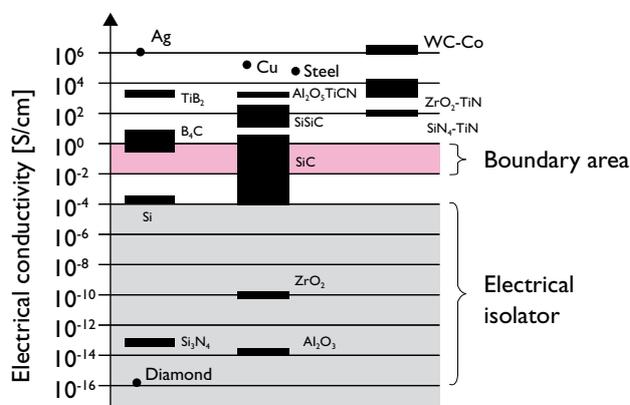
Figure 4. Overview of materials with their electrical conductivity.
