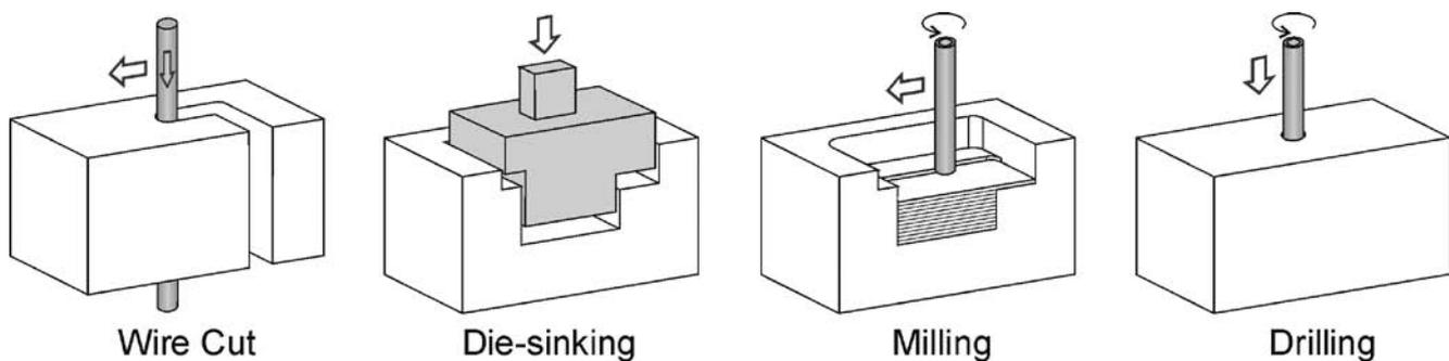
Figure 2. Most commonly used configurations of (micro-) EDM.
