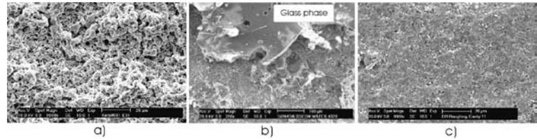
Figure 6. Various material removal mechanisms of  $\mu$ -EDM on  $Si_3N_4$ -TiN, as explained in the text.
