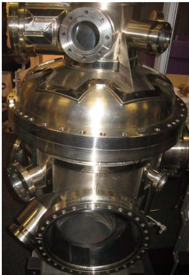
Figure 11. A welded stainless steel recipient, fabricated by D&M.
