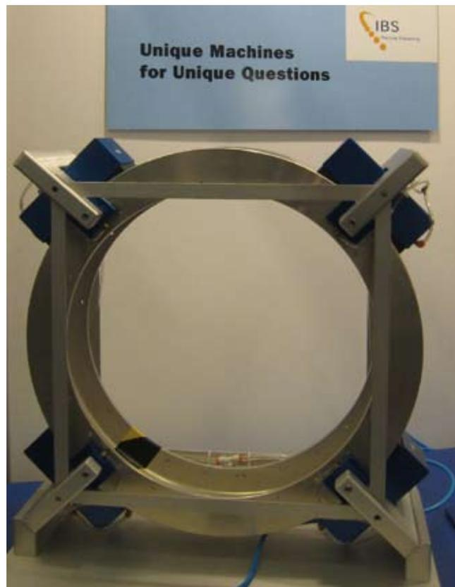
Figure 6. A ring rotating in air bearings made from New Way's porous carbon.
