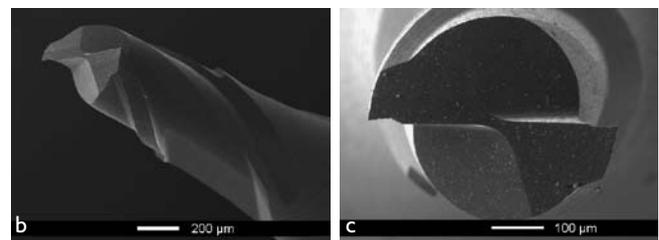
Figure 1. Geometry of a micro square endmill.
