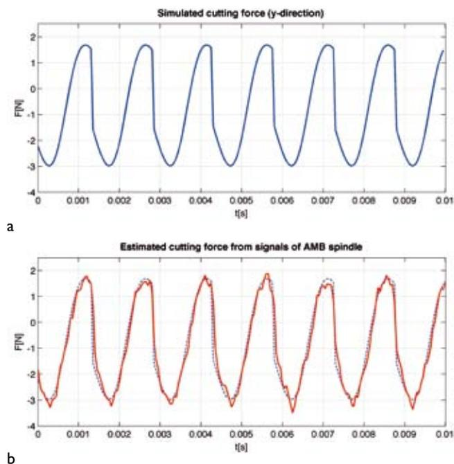
Figure 9. Simulation results of cutting force estimation from the signals of the AMB spindle. Results are only shown for one direction.
