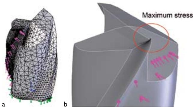
Figure 3. Study of tool geometry by FEM.
