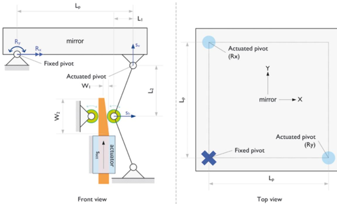
Figure 3. Tip-tilt mechanism concept.
