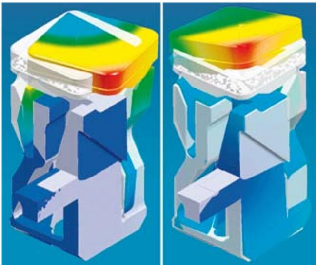
Figure 6. On the left the first resonant mode (355 Hz), on the right the second one (1,590 Hz).
