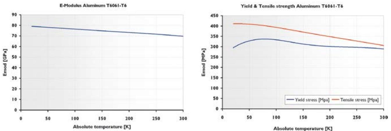
Figure 5. Aluminum T6061-T6 properties (E-modulus and yield/shear strength) against temperature.
