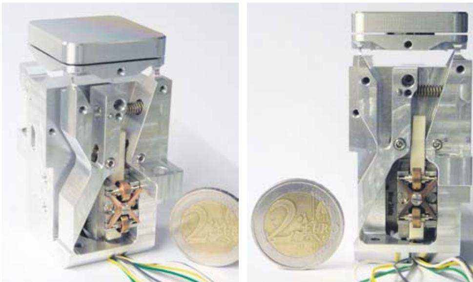
Figure 4. Two views of the realised tip-tilt mechanism.
