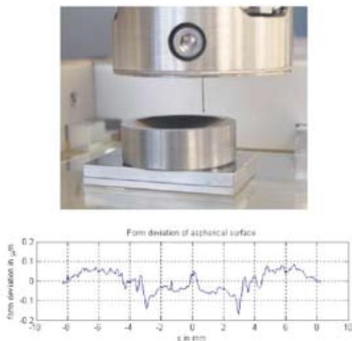
Figure 8. Aspheric mould measurement using the Triskelion probe.
