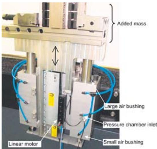
Figure 6. The Z-axis drive with weight compensation system.
