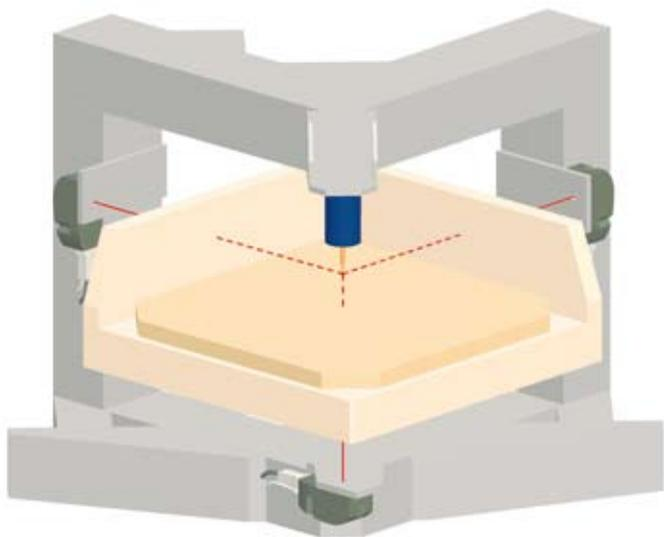
Figure 2. The 3D Abbe principle of the Isara 400 CMM.
