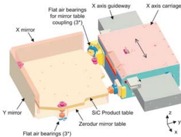
Figure 4. Floating mirror table and X-axis drive.
