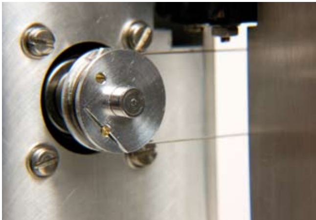
Figure 5. The motor pulley with the cable attached by means of steel soldered balls.
