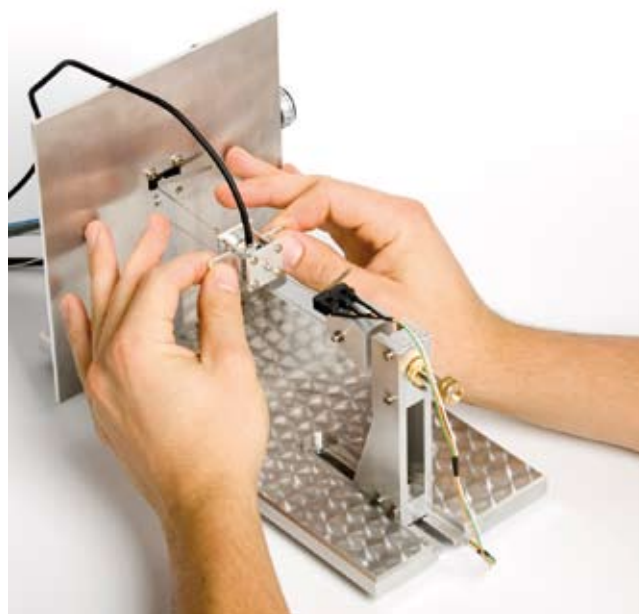
Figure 4. The epidural needle insertion simulator as used for the experiments. (Photo: Manon Eekhout)
