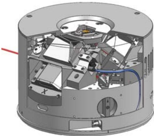
Figure 5. The new metrological AFM being developed at Eindhoven University of Technology. (Courtesy of TU/e)
