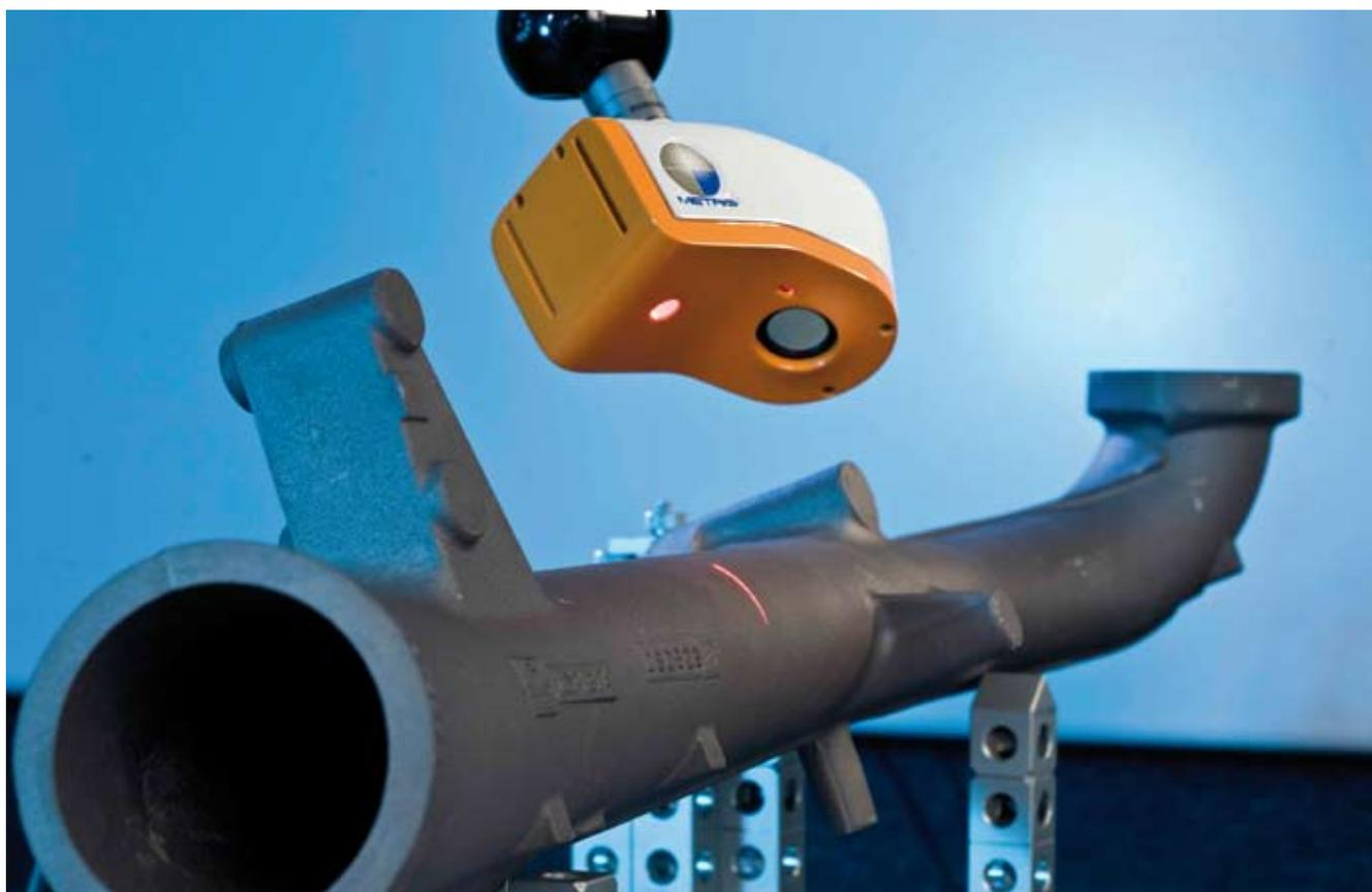
Figure 4. Laser scanner scanning a workpiece. The laser projecting the line is situated in the left part of the scanner, the lens and camera are in the right part. (Courtesy of Sirris)
