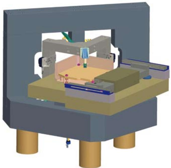
Figure 2. The new Isara 400 ultra-precision CMM being developed by IBS. (Courtesy of IBS Precision Engineering)
