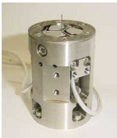
Figure 3. The IBS ultra-precision touch probe which will be used on the new Isara 400. (Courtesy of IBS Precision Engineering)
