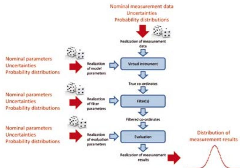
Figure 1. Schematic representation of a Monte-Carlo uncertainty calculation. (Courtesy of VSL)
