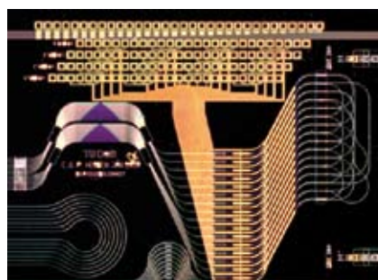
Figure 2. An optical crossconnect (OXC) chip that can switch four wavelength channels independently from two input waveguides to two output guides. It integrates two
