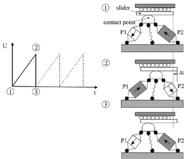
Figure 12. Working principle of the pulse-drive mode.
