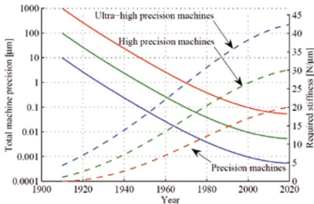
Figure 2. Taniguchi curves (solid lines) and extended Taniguchi curves (dashed lines) to describe trends for required machine accuracy and stiffness.
