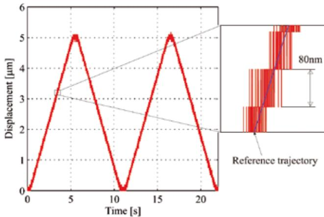
Figure 11. Tracking performance in the resonant-drive mode for a speed of 1 μm/s when a lead-lag controller is implemented.
