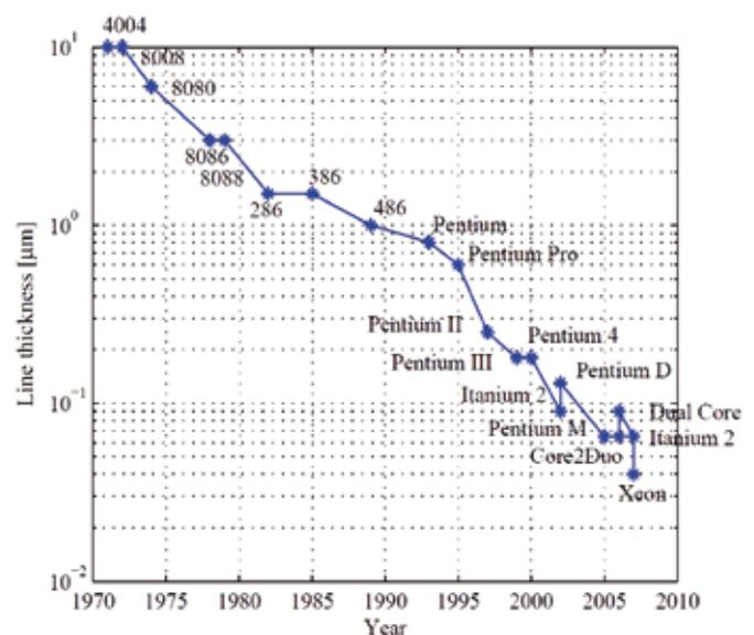
Figure 1. Evolution of the circuit line thickness of Intel processors (data collected from [www.intel.com](http://www.intel.com)).
