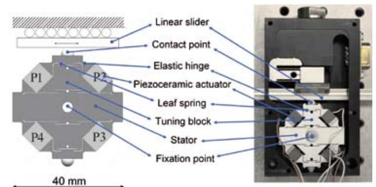
Figure 3. Schematic drawing and photograph of the linear piezoelectric Leuven motor.
