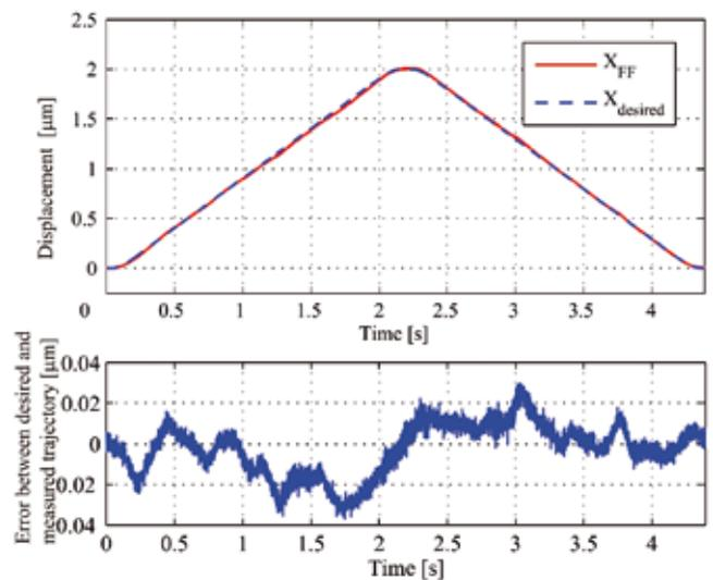
Figure 5. Comparison between measured, open-loop slider displacement and desired displacement for tracking a  $1 \mu\text{m/s}$  trajectory with the direct-drive mode (top). The bottom plot shows the error between desired and measured trajectory.
