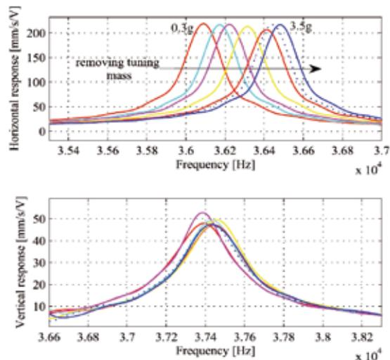
Figure 9. Variation of the horizontal (above) and vertical (below) eigenmode when changing the tuning mass.
