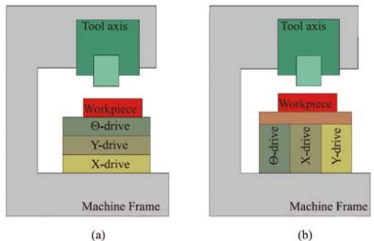
Figure 16. Schematic layout of (a) a classic positioning system, and (b) a parallel system with integrated drive-bearing function.
