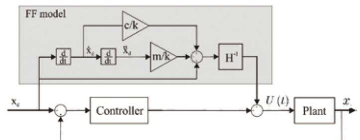
Figure 6. Schematic diagram of the controller for the direct-drive mode.
