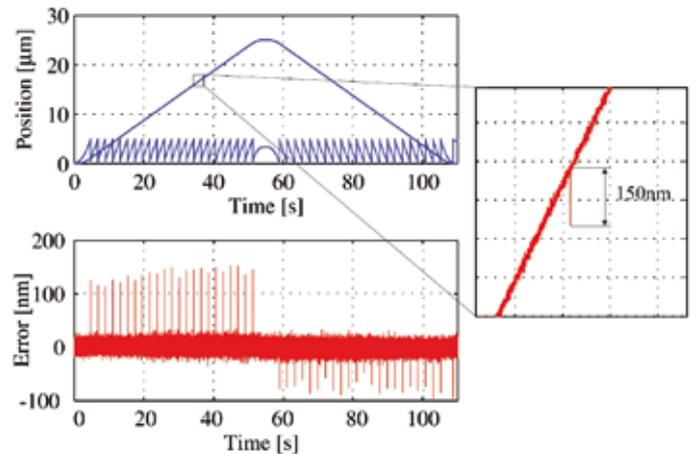
Figure 13. Experimental example of trajectory tracking with the pulse-drive mode.
