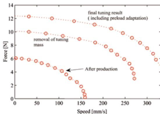
Figure 10. Influence of tuning on the traction-speed characteristic of the Leuven motor.
