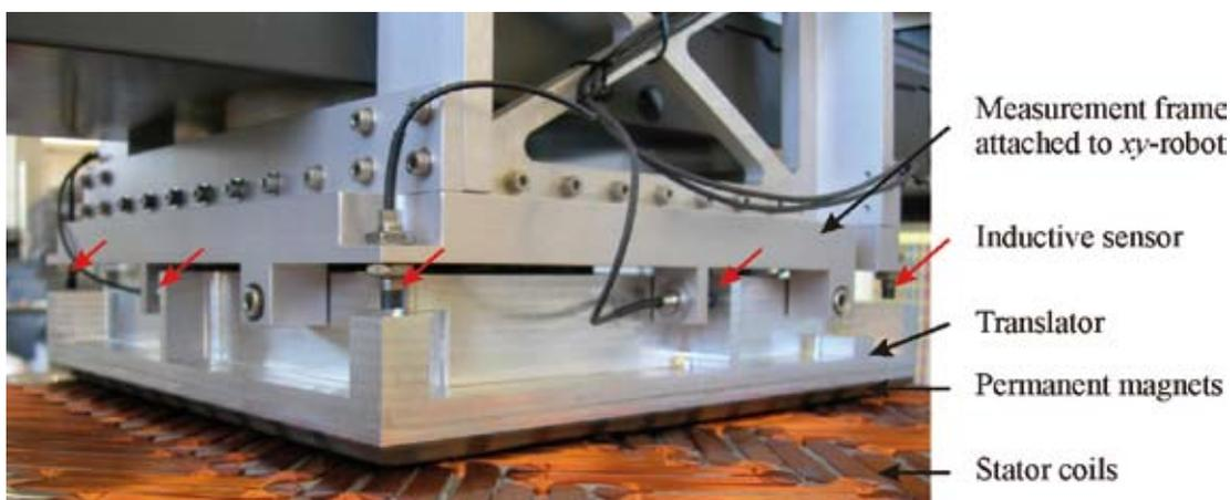
Figure 2. Herringbone Pattern Planar Actuator and measurement frame
